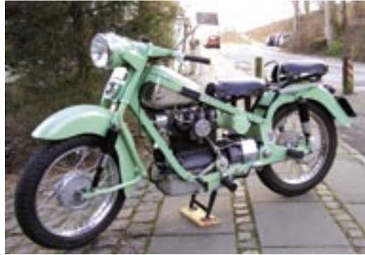
C, which was made from 1934 to 1959. The engine is an OHC inline 4-cylinder of 746 cc, generating a leisurely 22 hp, and known as a “bumblebee” from its exhaust note. Valve gear was exposed until the very latest models, which is not as messy as you might expect, says Nyborg. It's nothing like a Norton International, which required the rider wear oilcloth pants.
